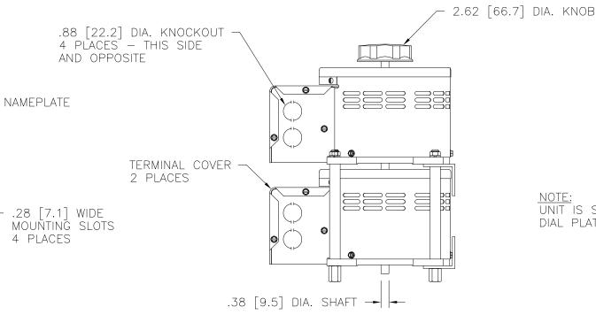
UNIT IS SUPPLIED WITH A 3.75 [95.2] DIA. 0-100 GRADUATED DIAL PLATE FOR PANEL MOUNTING.
