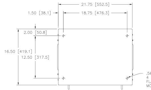
.56 [14.3] DIA. HOLE 4 PLACES ON BOTTOM FLANGES FOR CUSTOMER MOUNTING
