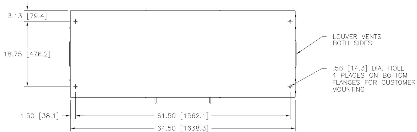
EACH PHASE OF THE REGULATOR COMPRISES A MOTOR-DRIVEN VARIABLE AUTOTRANSFORMER, A BUCK-BOOST FIXED RATIO TRANSFORMER, AND A MANUAL RAISE/LOWER SWITCH. THE MICROPROCESSOR CONTROLLER AUTOMATICALLY POSITIONS EACH OF THE AUTOTRANSFORMERS TO HOLD THE OUTPUT VOLTAGE OF EACH PHASE CONSTANT. A RS-232 INTERFACE IS PROVIDED FOR REMOTE OPERATION AND MONITORING.
